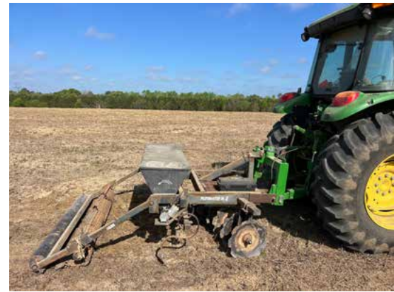
Seed spreader attachment for a tractor used in planting a large pollinator meadow at a private property near Waynesboro. Photo by Jesse Kamps
